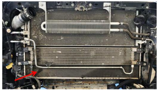
NOTE: The spring clamp from the stock transmission cooler line will be reused, remove from the stock line and set aside.
