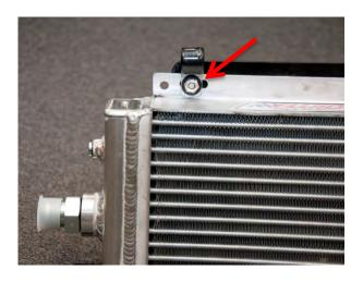
5. Loosely install the ¼ inch loop clamp in the correct hole, as shown. Leave the loop clamp loose to slip the hose through later.
