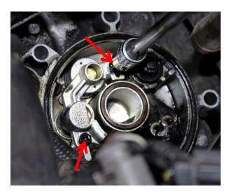
Remove the 2 Torx head bolts holding the stock bypass/anti-drain back assembly in place.
