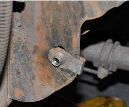
5. Mount the oil filter bracket on the truck using the stock hardware.
