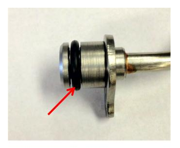
18. Reinstall the turbo oil feed line.
