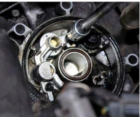
15. Install two #12 JIC 0° fittings into the Half Kit adapter.
