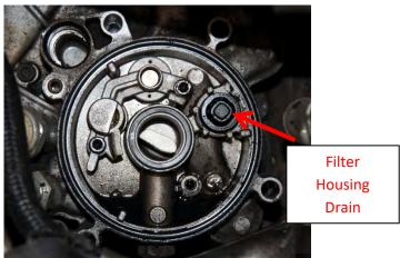
16. Install the Half Kit adapter where the stock oil filter housing was placed.
