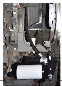
2. Install the hose clamp and adjustment strap to the core support.
