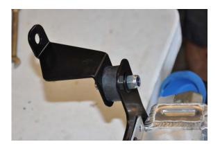
8. Install the support bracket, vibration-damping mount, and hardware to the oil cooler bracket.
