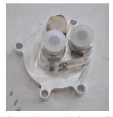
WARNING: When installing the Half Kit adapter, make sure the step on the bottom of the adapter is placed on the filter housing drain. Once the adapter is resting on the housing DO NOT SPIN OR TWIST IT. If the filter housing drain is broken, oil will not flow properly through the oiling system AND SEVERE ENGINE DAMAGE MAY RESULT.
