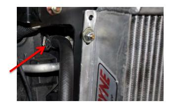
13. Connect new transmission cooler line to the correct port on the radiator using the stock spring clamp. Trim the hose to fit if necessary.
