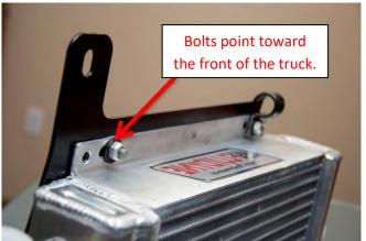
7. Remove the bolt on the core support as shown:
