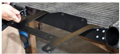
NOTE: Do not over-tighten. Stripping the screws will cause the bracket to be loose.
