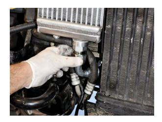
5. Take the 51" Hose #3 from the OIL IN port on the half kit adapter; route it over the air inlet tube, where it connects to the turbo, then under the air inlet tube, where it connects to the air filter box. Continue routing under the CAC pipe on the passenger side out to the front of the truck where the CAC pipe connects to the CAC. Attach the 45° hose end to the #12 JIC 90° fitting on the oil cooler.
