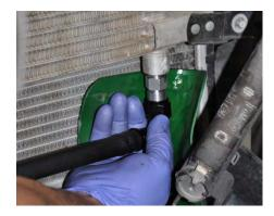
2. Route the hose along the bottom of the transmission cooler and behind the hose connected to the opposite side of the cooler. Secure the hose with the cable tie provided.
