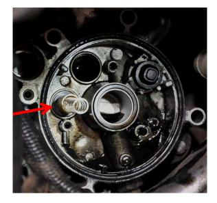
13. Place the bypass piston with the new provided spring back into the housing.
